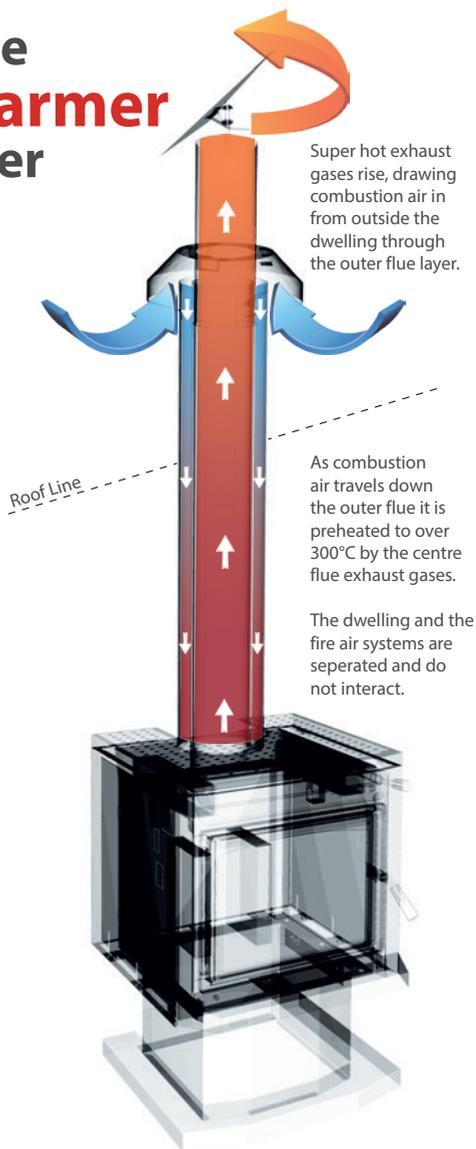
Combustion air is drawn from outside the home, down the outer section of the flue system.
